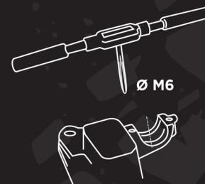
GB: Some brake and clutch pumps "MODEL YEAR 2014" may have the hole (for to the additional screw M6X12) with an incomplete thread. In this case, finish the thread using a M6 screw tap.
